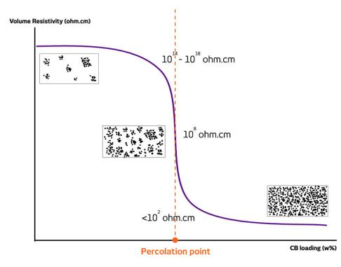
Percolation describes the contact between carbon black particles. At certain carbon black loading level the carbon black particles loose the direct contact between each other and the resistance increases dramatically. This point is called percolation point. Over the percolation point, the change in conductivity is very fast.
