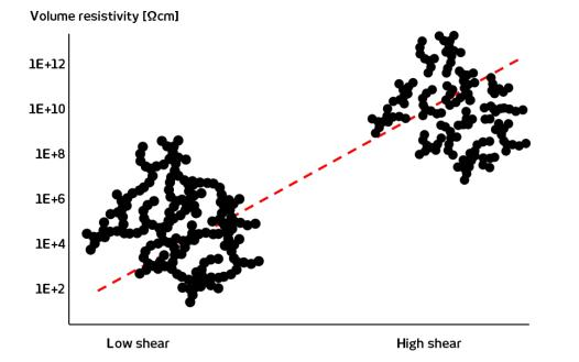
High shear forces often lead to breakage in carbon black network. This results in higher resistance of the moulded parts.
