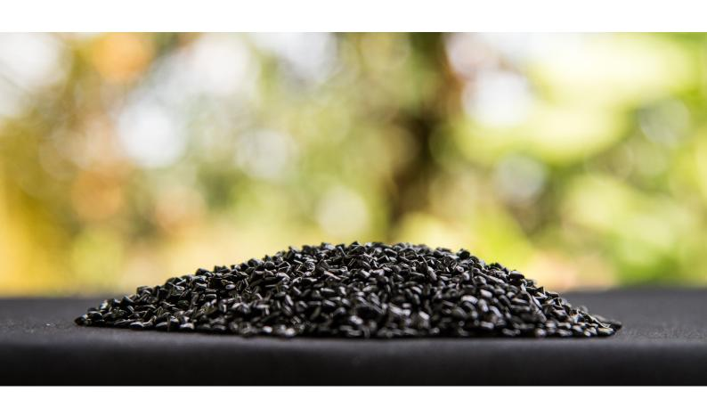
Unlike plastics in general, conductive plastics have the ability to conduct electricity. When grounded, conductive plastics remain at zero potential and do not accumulate static electricity. Premix's conductive PRE-ELEC® compounds offer a wide variety of solutions with applications ranging from precise pipette tips and sophisticated smart textile components to bigger articles, such as FIBC used in the transportation and storage of hazardous goods.
